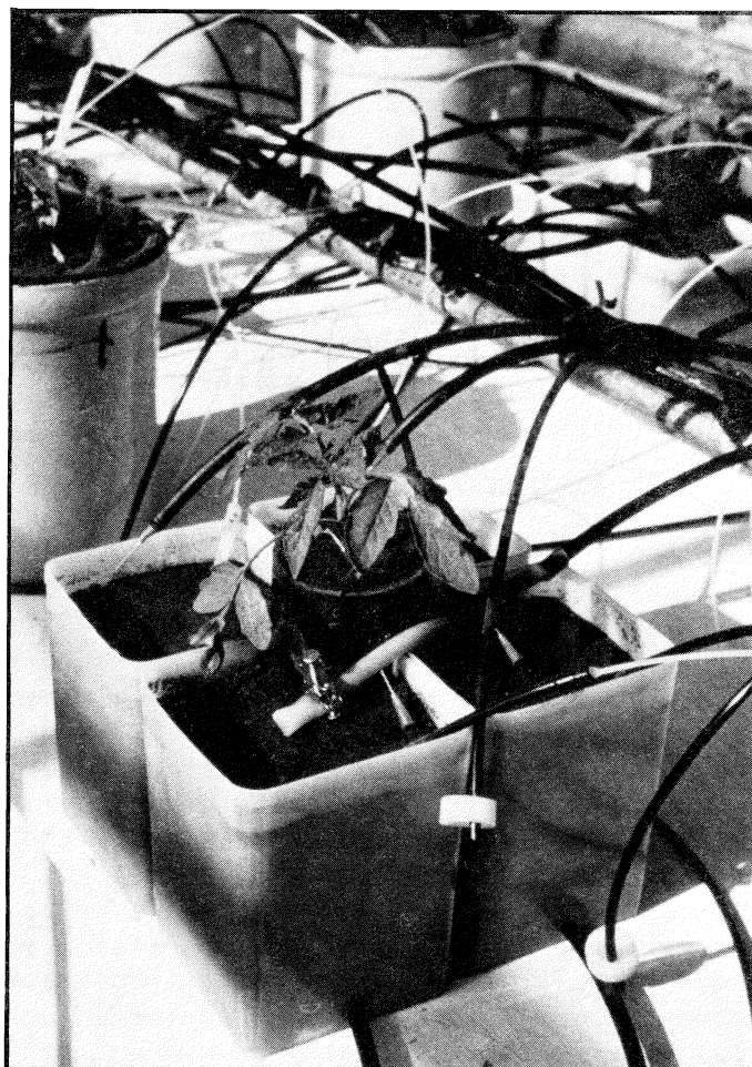
Apparatus for imposing split-root treatments.
