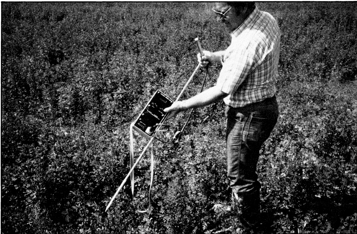
Instrument used to measure soil salinity distribution across fields.
