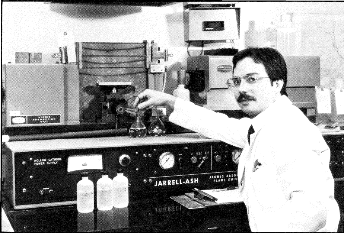
Atomic adsorption spectrophotometer being used for analysis of trace elements.
