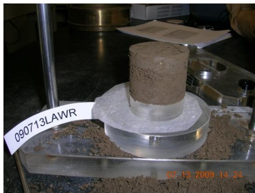
Fig. 1A Moist soil sample after trimming. Fig. 1B Soil sample mounted in the shearing device.
