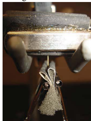
Fig. 2B Root segment in clamp
