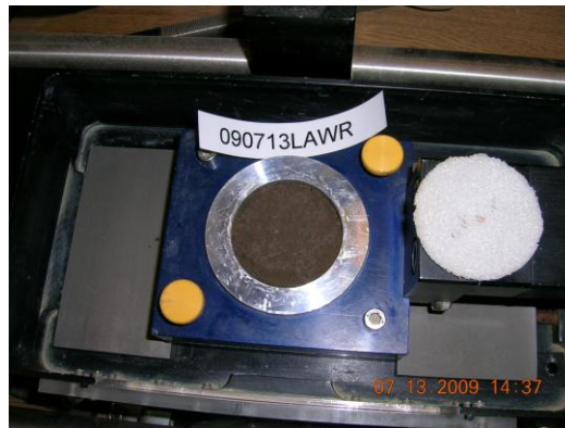
Fig. 1A Moist soil sample after trimming. Fig. 1B Soil sample mounted in the shearing device.
