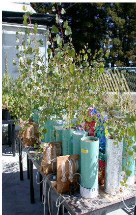
Fig. 1. Preparation for trapping CO 2 respired from the soil and rhizosphere. The pale blue material coating some of the pots is flexible silicone rubber, designed to isolate the soil gases from the ambient atmosphere.
